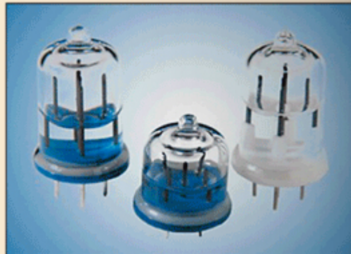
Figure 5. The SP5000 dual-axis electrolytic tilt sensor has an angular measurement range of \pm 60^\circ , repeatability of \pm 0.03^\circ , and an operating temperature range of -40^\circ\text{C} to 80^\circ\text{C} . It has no moving parts, a symmetrical pin design for easy PC board mounting, and is hermetically sealed.
